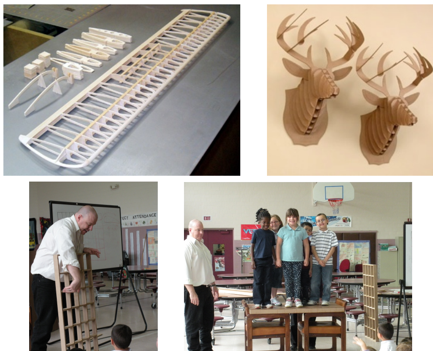
FIGURE 2.1. Three-dimensional objects constructed from two-dimensional components: airplane wing, Carboard Safari trophies, and the first author demonstrating the strength of torsion boxes with a little help from some of his friends.
