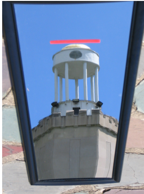
FIGURE 6.5. Citing the Carillon Tower using mirror reckoning. Note the piece of tape at the top the image of the dome.
